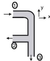
$$\begin{aligned}v_1 &= 6 \text{ m/s} & p_1 &= 4.8 \text{ kPa} \\v_2 &= v_3 = 3 \text{ m/s} & p_2 &= p_3 = 0 \\A_1 &= A_2 = A_3 = 0.20 \text{ m}^2\end{aligned}$$
