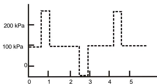
At  $t = 1.5$  s high pressure wave will have travelled to reservoir and static wave will be travelling toward valve.
