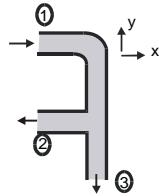
$$\begin{aligned}\dot{m}_1 &= 12 \text{ lbm/s} \\ \dot{m}_2 &= \dot{m}_3 = 6 \text{ lbm/s} \\ A_1 &= A_2 = A_3 = 5 \text{ in}^2 \\ p_1 &= 5 \text{ psig} \\ p_2 &= p_3 = 0\end{aligned}$$
