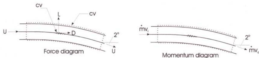
The force diagram shows a lift force and drag force produced by the airfoil and act on the control surface. There is no net pressure force on the outer surface since the pressure is constant. The momentum diagram shows an inflow and outflow of momentum. From continuity, the mass flow rate in is equal to the mass flow rate out. The sum of the forces in the x-direction is
