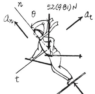
**Kinematics:** The speed of the skier can be determined using  $v dv = a_t ds$ . Here,  $a_t$  must be in the direction of positive  $ds$ . Also,  $ds = \sqrt{1 + (dy/dx)^2} dx = \sqrt{1 + \frac{1}{100}x^2} dx$
