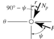
$$\tan(\psi) = \frac{r}{\frac{dr}{d\theta}} = \frac{ae^{b\theta}}{ab e^{b\theta}} = \frac{1}{b} \quad \psi = \tan^{-1}\left(\frac{1}{b}\right) \quad \psi = 84.29^\circ \quad \text{Ans.}$$
