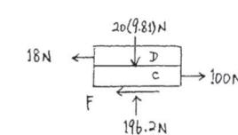
Check slipping between *D* and *C*.
