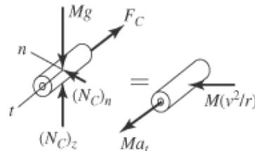
$$d = \int_{v_I}^0 \frac{v}{a_t(v)} dv \quad d = 0.581 \text{ m} \quad \text{Ans.}$$
