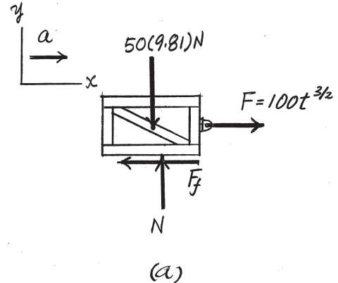
**Kinematics:** Using the result of **a** and integrating the kinematic equation  $dv = a dt$  with the initial condition  $v = 0$  at  $t = 1.567$  as the lower integration limit,
