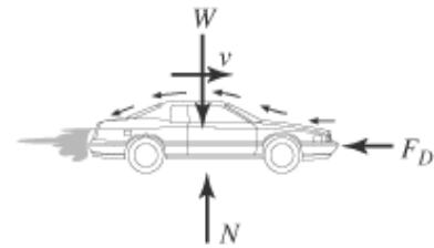
$$\text{Find distance } a = v \frac{d}{dx} v = \frac{-k}{m} v$$
