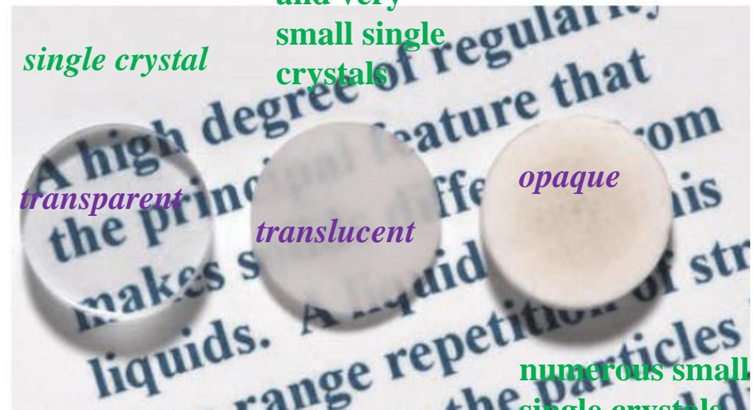
Three thin disk specimens of aluminium oxide
