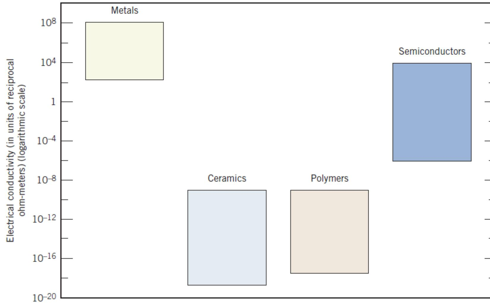
Bar chart of room-temperature electrical conductivity ranges for metals, ceramics, polymers, and semiconducting materials.
