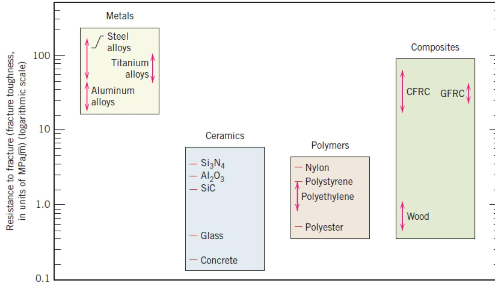
Bar chart of room-temperature resistance to fracture (i.e., fracture toughness) for various metals, ceramics, polymers, and composite materials.
