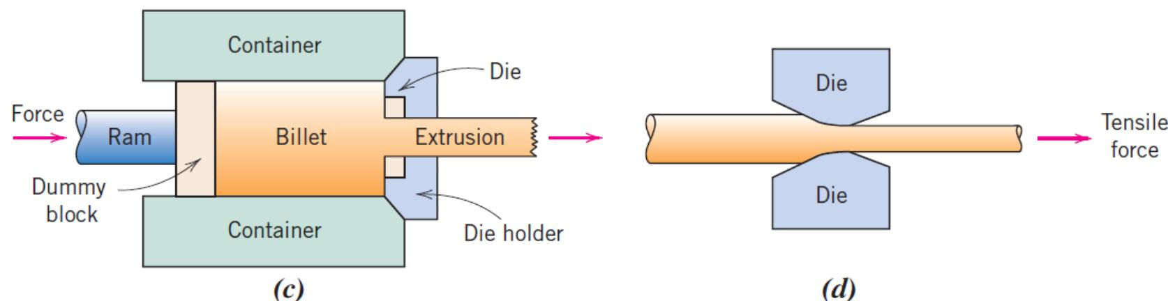
Metal deformation during (a) forging, (b) rolling, (c) extrusion, and (d) drawing
