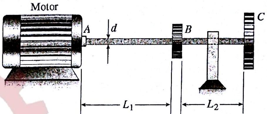
**Problem.9 (3- points)** For the previous problem, if  $d=60$  mm, then the angle of twist between the motor and gear *C* is:
