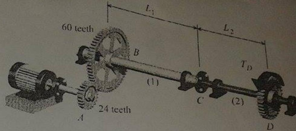
$$20 \text{ kW} / w = 400 \text{ rpm} / d_1 = 50 / G_1 = 28 \text{ GPa} / \delta_1 = 1200 /$$
