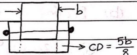
(a) Find the minimum diameter Required of the bolt?
