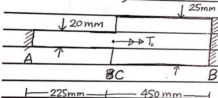
(a) if  $T_{allow} = 43 \text{ MPa}$  Find  $T_{o(max)} = ??$
