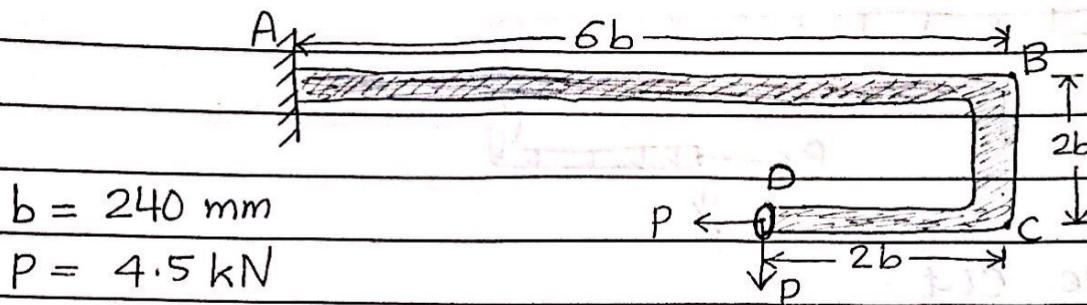
(a) Find the minimum diameter if  $\sigma_{\text{allow}} = 110 \text{ MPa}$ .
