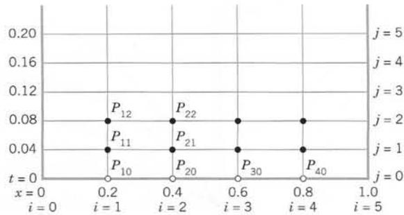
Fig. 467. Grid in Example 1
