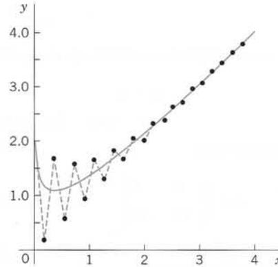
Fig. 451. Euler method with  $h = 0.18$  in Example 4
