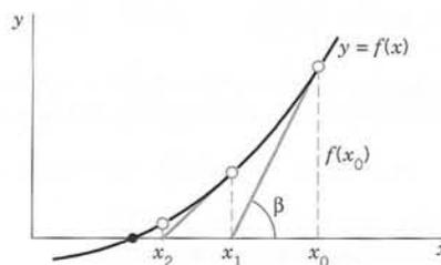
Fig. 425. Newton's method
