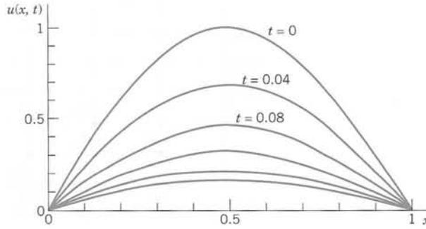
Fig. 468. Temperature distribution in the bar in Example 1
