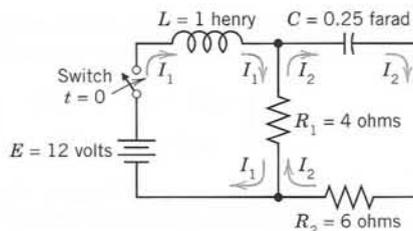
Fig. 78. Electrical network in Example 2
