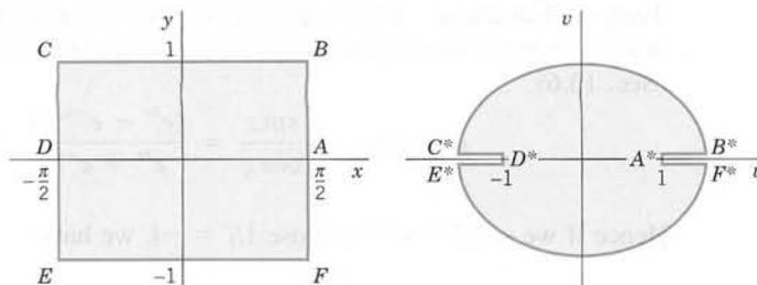
Fig. 389. Mapping by  $w = \sin z$
