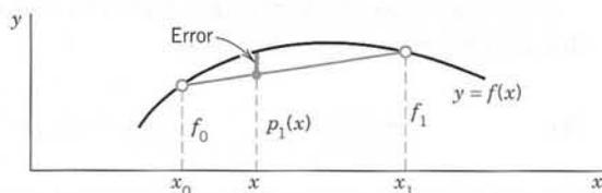
Fig. 428. Linear interpolation
