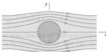
Fig. 412. Flow around a cylinder (Example 2)
