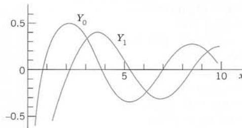
Fig. 109. Bessel functions of the second kind  $Y_0$  and  $Y_1$ .
