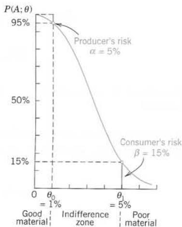
Fig. 539. OC curve, producer's and consumer's risks
