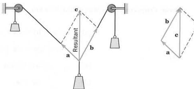
Fig. 169. Resultant of two forces (parallelogram law)
