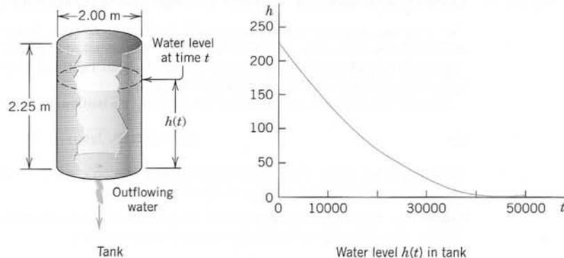
Fig. 11. Example 5. Outflow from a cylindrical tank ("leaking tank"). Torricelli's law
