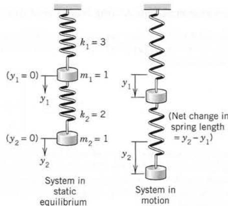
Fig. 159. Masses on springs in Example 4
