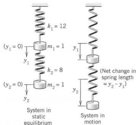
Fig. 80. Mechanical system in Team Project 16
