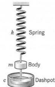
Fig. 35. Damped system
