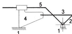
2. Use equation 2.1c to determine the *DOF* (mobility). There are 5 links, 4 full pin joints, 1 full sliding joint, and 1 half joint (at the interface between the hacksaw blade and the pipe being cut).
