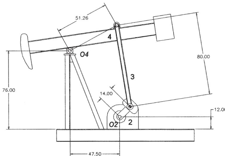
This is a basic fourbar linkage. The input is the 14-in-long crank (link 2) and the output is the top beam (link 4). The mobility (DOF) is found using equation 2.1c (Kutzbach's modification):
