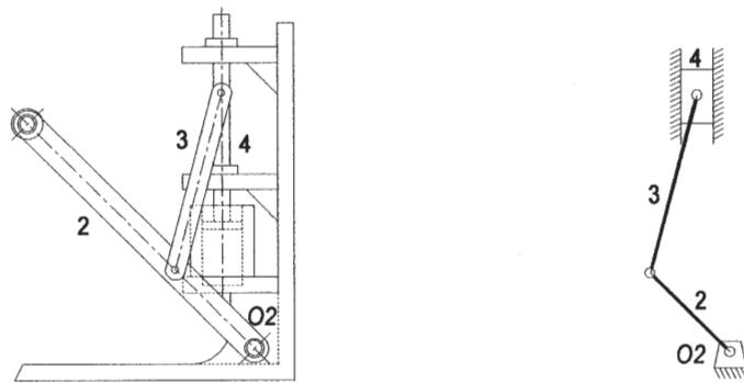
2. Use equation 2.1c to determine the *DOF* (mobility). There are 4 links, 3 full pin joints, 1 full sliding joint, and 0 half joints. This is a fourbar slider-crank.
