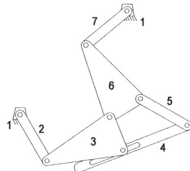
2. Use rule 3 on page 42, which states: "Removal of a link will reduce the DOF by one." One way to do this is to remove link 7 such that link 6 pivots on the fixed pin attached to the ground link (1). We now have mobility:
