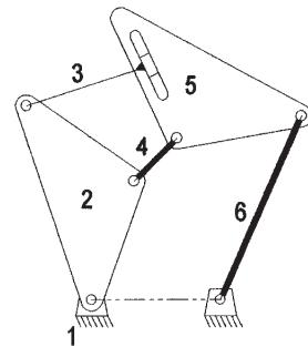
3. To get the half joint, use rule 4 on page 42, which states: "The combination of rules 2 and 3 above will keep the original DOF unchanged." One way to do this is to remove link 6 (and its two nodes) and insert a half joint between links 5 and 1.
