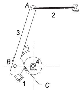
2. Use equation 2.1c to determine the *DOF* (mobility). There are 4 links, 3 full pin joints, 1 half pin-in-slot joint (at *B*), and 1 half joint (at the interface *C* between the two gears, shown above by their pitch circles). Links 1 and 3 are ternary.
