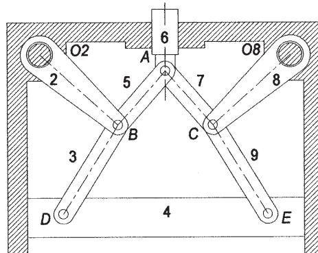
The result is that this mechanism seems to be a structure. By splitting it into mirror halves about the vertical centerline the mobility is found to be 1. Subtract the 3 redundant links and their 5 (6 minus the joint at A) associated joints to determine the mobility of the mechanism.
