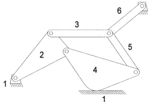
2. Use rule 2 on page 42, which states: "Any full joint can be replaced by a half joint, but this will increase the DOF by one." One way to do this is to replace one of the pin joints with a pin-in-slot joint such as that shown in Figure 2-3c. Choosing the joint between links 2 and 4, we now have mobility:
