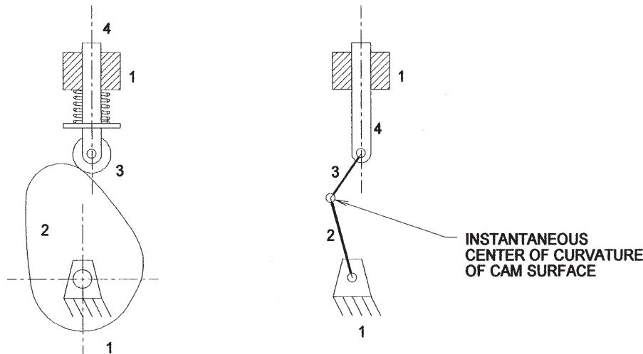
2. Use equation 2.1c to determine the *DOF* (mobility) of the original mechanism. There are 4 links, 2 full pin joints, 1 full sliding joint, 1 pure rolling joint and 0 half joints.
