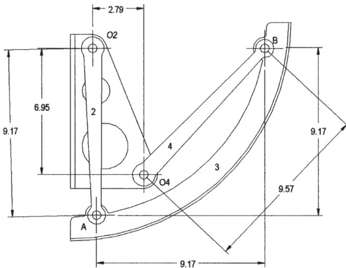
This is a basic fourbar linkage. The input is the link 2 and the output is link 4. The mobility (DOF) is found using equation 2.1c (Kutzbach's modification):
