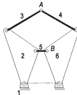
2. Use rule 1 on page 42, which states: "Revolute joints in any loop can be replaced by prismatic joints with no change in DOF of the mechanism, provided that at least two revolute joints remain in the loop." One way to do this is to replace pin joints at A and B with translating full slider joints such as that shown in Figure 2-3b.
