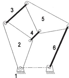
2. To get the sliding full joint, use rule 1 on page 42, which states: "Revolute joints in any loop can be replaced by prismatic joints with no change in DOF of the mechanism, provided that at least two revolute joints remain in the loop." One way to do this is to replace pin joint links 3 and 5 with a translating full slider joint such as that shown in Figure 2-3b.
