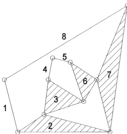
The mechanism shown in Figure P2-5b is the same eightbar isomer as that depicted schematically above.
