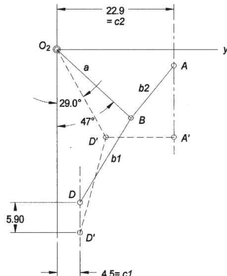
5. Use equations 4.17 and 4.16b to determine the displacement of  $D'$  with respect to  $O_2$ .
