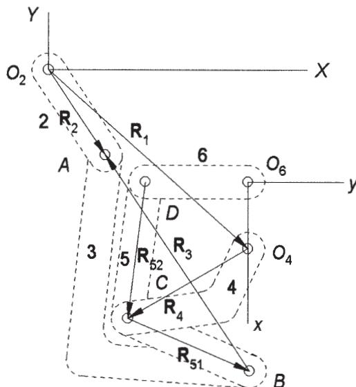
$\mathbf{R}_1 + \mathbf{R}_4 + \mathbf{R}_{51} + \mathbf{R}_3 - \mathbf{R}_2 = 0$ . In this equation the unknowns are  $\theta_3$  and  $\theta_2$ . Following the method of Section 4.5, substitute the complex number notation for each position vector and separate the resulting equations into real and imaginary parts:
