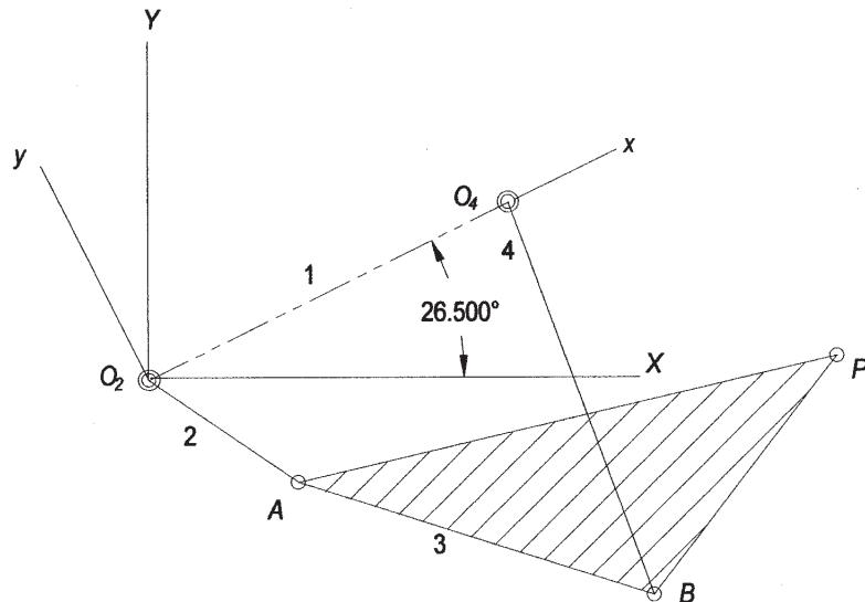
2. Define one revolution of the input crank:  $\theta_2 := 0 \cdot \text{deg}, 2 \cdot \text{deg}..360 \cdot \text{deg}$
