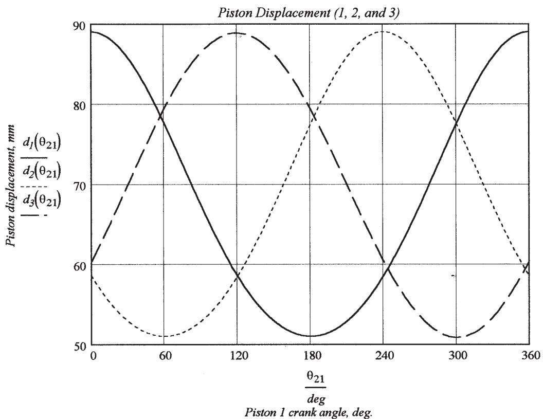
The solid line is piston 1, the dotted line is piston 2, and the dashed line is piston 3.
