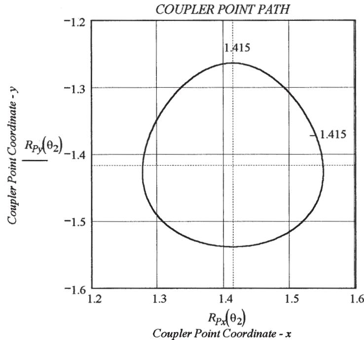
6. Replot, transforming the coupler path to 0,0 and plot the path of point A.
