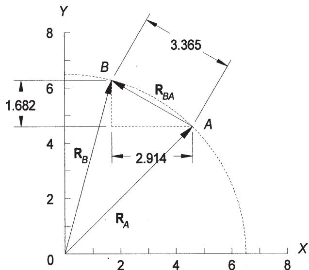
On the layout above the  $X$  and  $Y$  components of  $\mathbf{R}_{BA}$  are equal to the real and imaginary components calculated, confirming that the calculation is correct.
