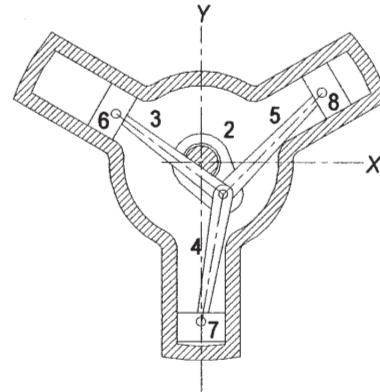
4. For each piston (slider) the crank angle is measured counter-clock-wise from the centerline of the piston, which goes through the  $O_2$  in all cases. Thus, when the crank angle for piston 1 is 0 deg, it is 120 deg for piston 2 and 240 deg for piston 3. Thus, the crank angles for pistons 2 and 3 are
