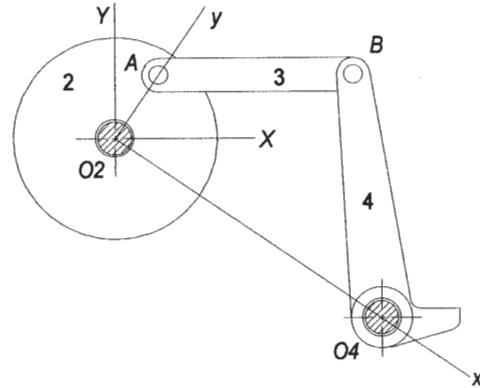
5. Determine the values of the constants needed for finding  $\theta_3$  from equations 4.11b and 4.12.
