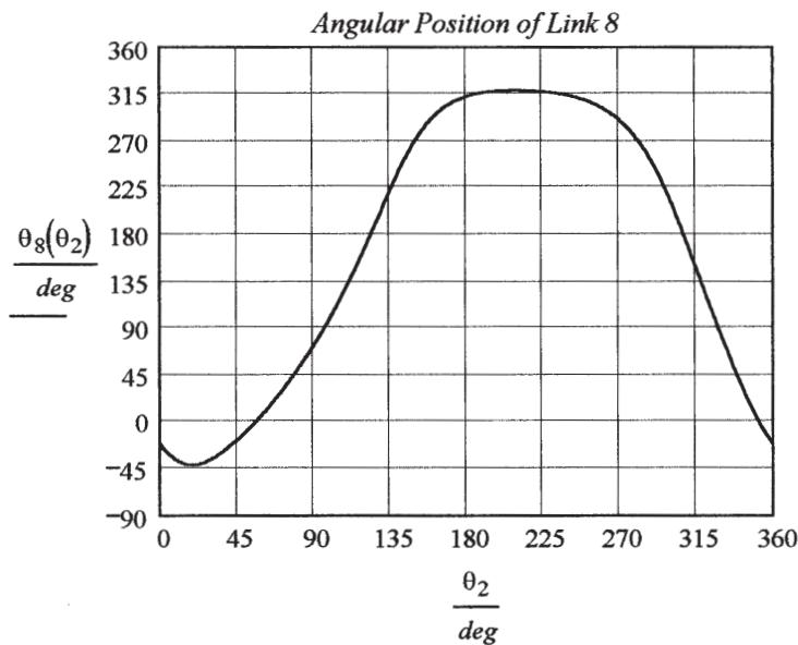
The graph shows that link 8 rotates 360 deg between  $\theta_2 = 19$  deg and  $\theta_2 = 209$  deg.
