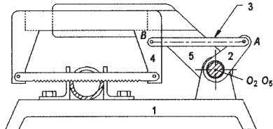
**Assumptions:** The arm that guides the slider (hacksaw blade carrier) remains horizontal throughout the stroke.
