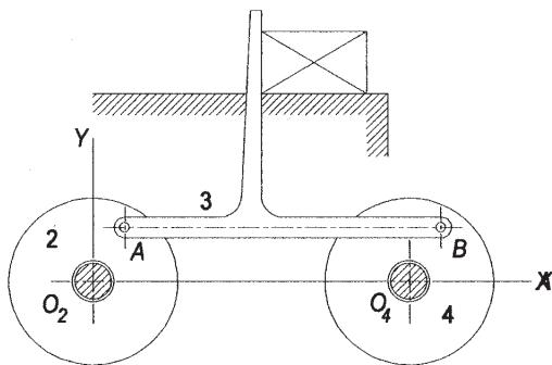
1. This is a special-case Grashof mechanism in the parallelogram form (see Figure 2-17 in the text). As such, the coupler link 3 executes curvilinear motion and is always parallel to the ground link 1. Thus, the total angular motion of link 3 as crank 2 makes one complete revolution is zero degrees.
