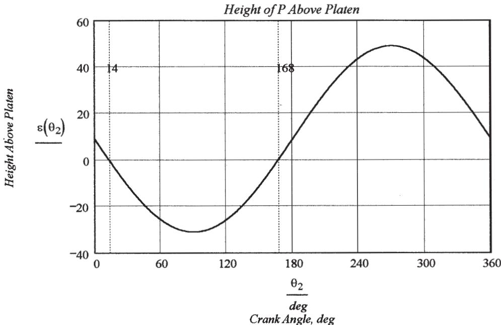
6. From the graph we see that the coupler point  $P$  is above the platen when the crank angle is greater than 168 deg and less than 14 deg. To find the horizontal stroke during that range of  $\theta_2$ , calculate the  $x$ -components of any point on the coupler, say point A, for those two crank angles and subtract them.
