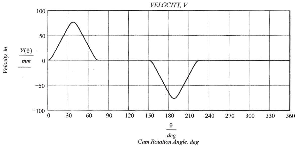
12. Write the complete global equation for the acceleration and plot it over one rotation of the cam, which is the sum of the four intervals defined above.
