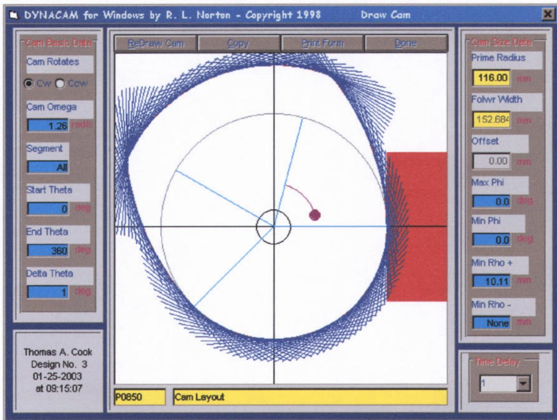
4. The minimum and maximum radius of curvature are shown in the figure above. The design has the following dimensions:
