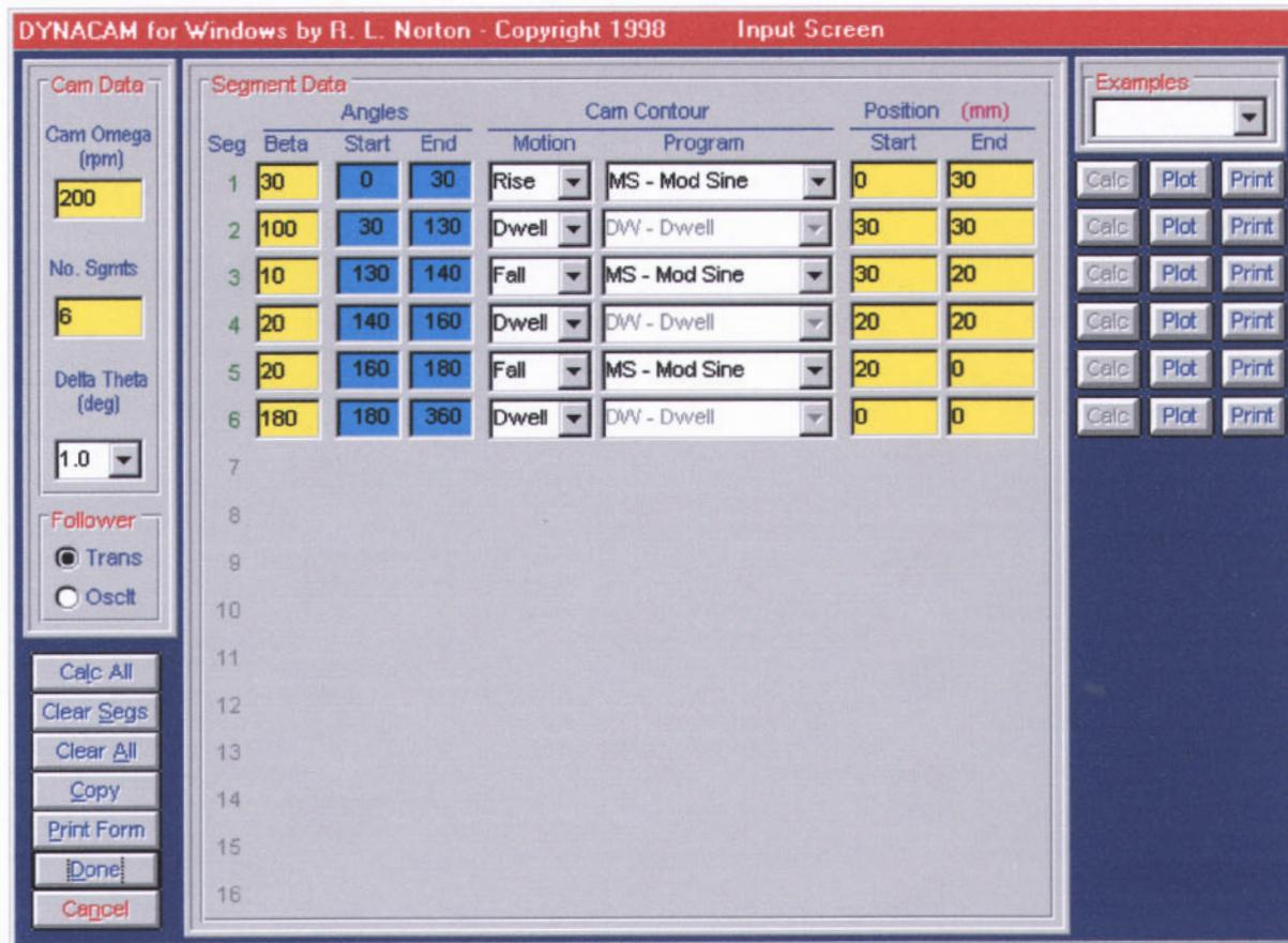
2. The cam was sized iteratively to balance the positive and negative extreme values of the pressure angle by varying the eccentricity and to reduce the maximum absolute pressure angle to 25 deg or less by increasing the prime circle radius. The resulting cam is shown below.
