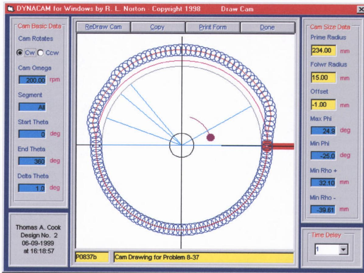
3. The minimum and maximum pressure angles and radius of curvature are shown in the figure above. The design has the following dimensions:
