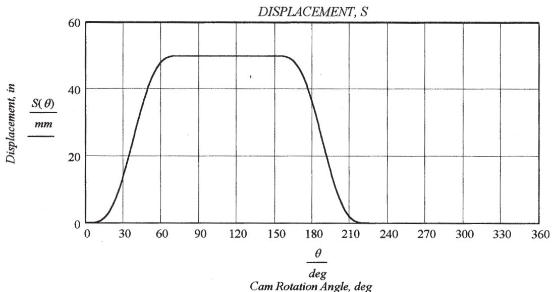
9. Write the complete global equation for the velocity and plot it over one rotation of the cam, which is the sum of the four intervals defined above.
