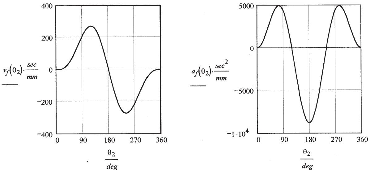
4. Determine the angular displacement, velocity, and acceleration of the arm, link 4.
