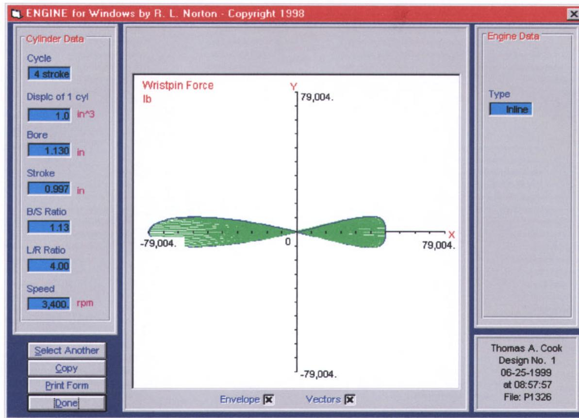
3. Enter the above data and the masses for part c into program ENGINE to determine the maximum value of the force on the wrist pin and to get the polar plot of this force.
