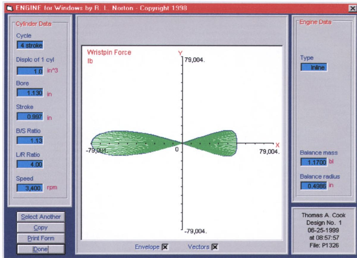
3. Enter the above data and the masses for part *c* into program ENGINE to determine the maximum value of the force on the wrist pin and to get the polar plot of this force.
