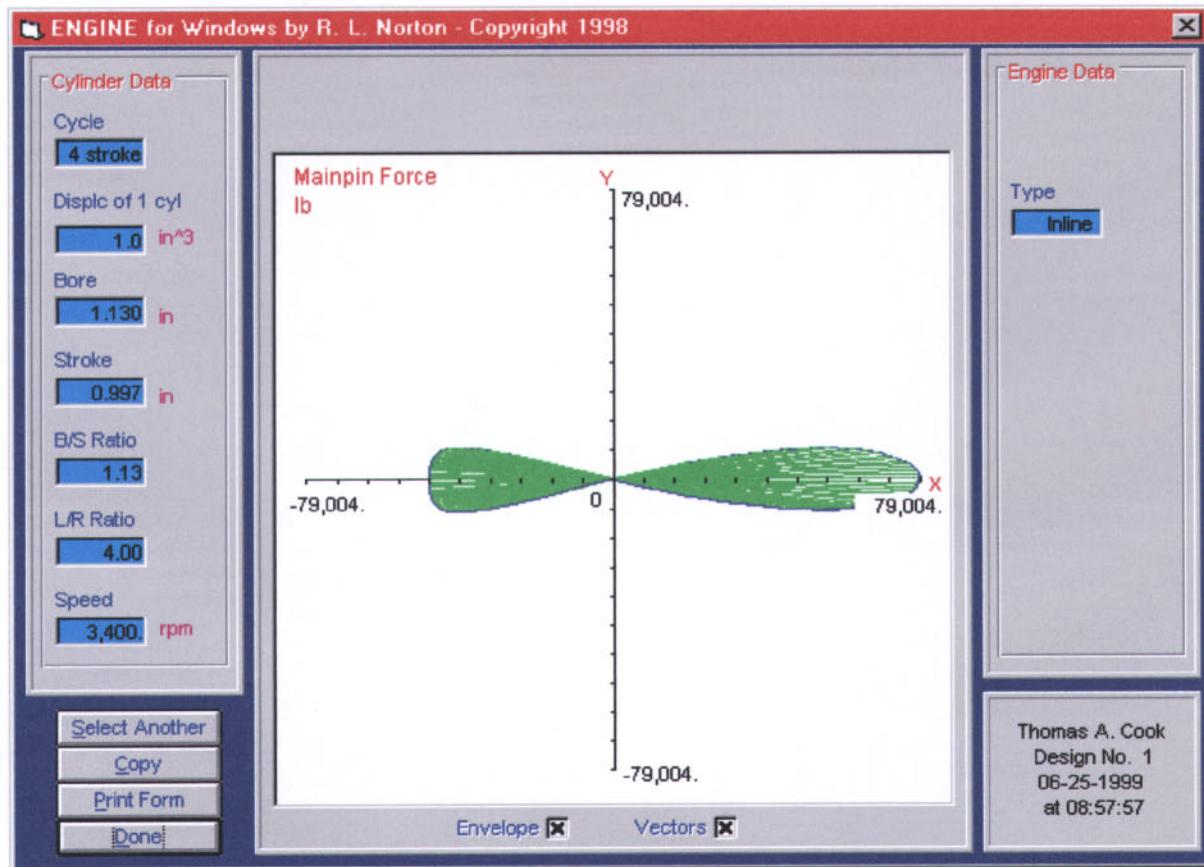
3. Enter the above data and the masses for part *c* into program ENGINE to determine the maximum value of the force on the main pin and to get the polar plot of this force.
