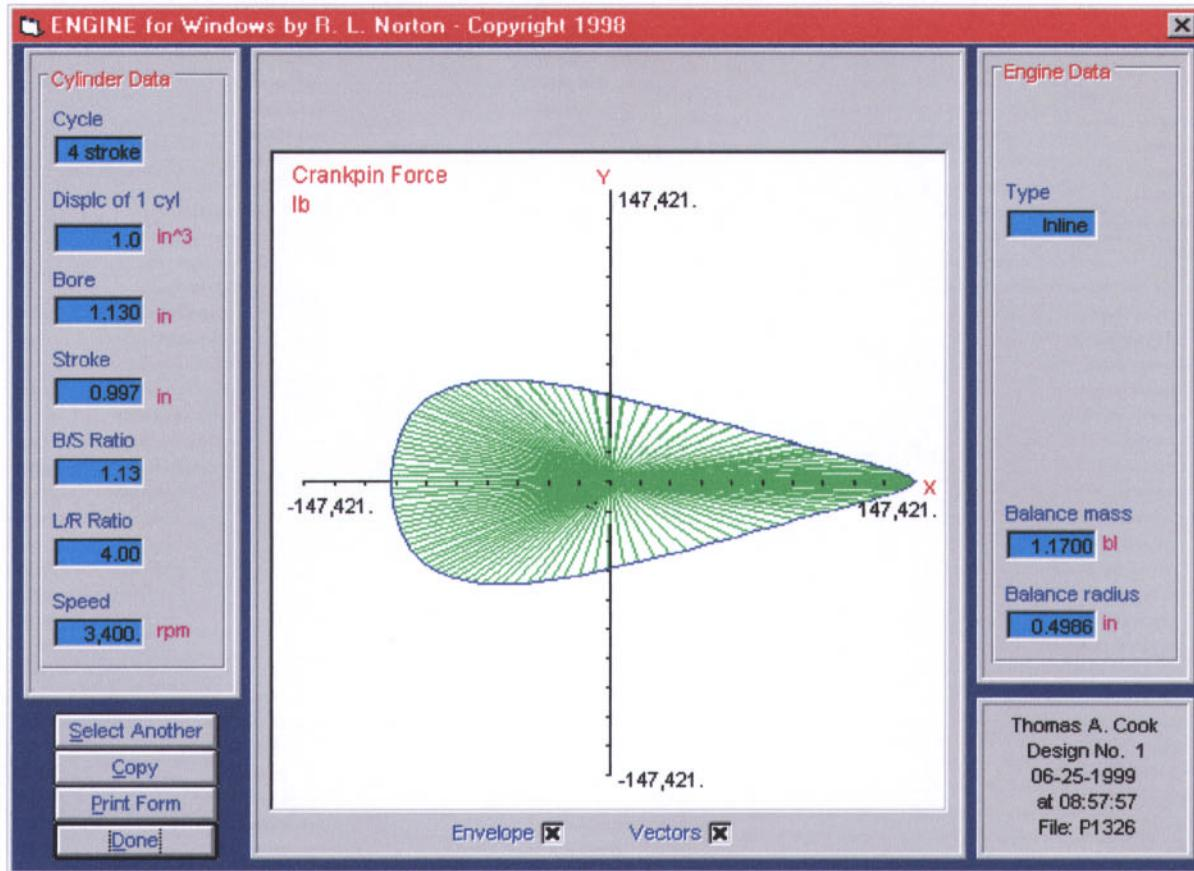
3. Enter the above data and the masses for part c into program ENGINE to determine the maximum value of the force on the crankpin and to get the polar plot of this force.
