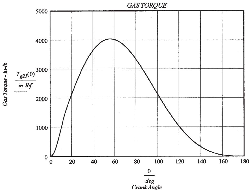
3. Integrate the gas torque over the range of crank motion (180 deg) to determine the energy delivered.
