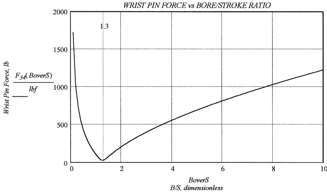
8. The graph shows that there is an optimum value of  $B/S$  that will minimize the wrist pin force, which in this case, is about  $B/S = 1.3$ . However, the optimum value is dependent on the other design choices (especially peak gas pressure) and can vary considerably from this value. The bore, stroke, and crank radius that would result from choosing this value are:
