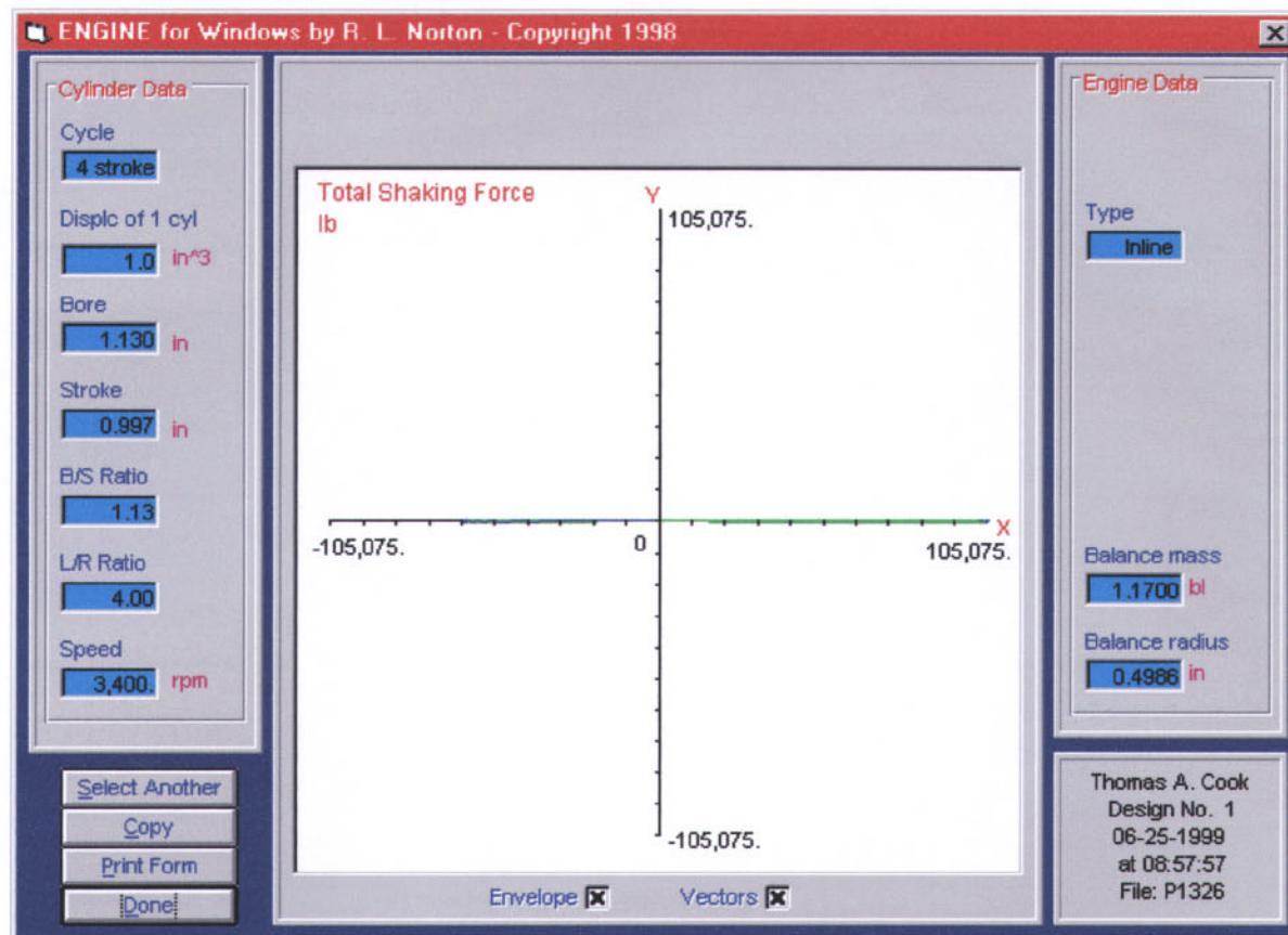
3. Enter the above data and the masses for part *c* into program ENGINE to determine the maximum value of the shaking force and to get the polar plot of this force.
