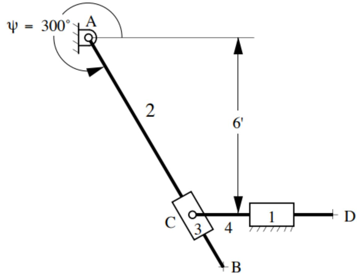
P5. In the mechanism shown, link 3 is perpendicular to link 2. Use the loop closure equation to find the acceleration of point C. The angular velocity of link 2 is constant and equal 100 rad/s CCW.
