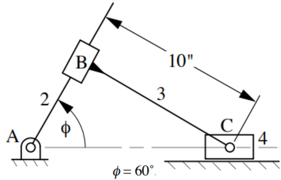
P4. For the mechanism shown, link 2 rotates with an angular velocity of 200 rad/s. use the loop closure equation to determine the angular velocity and acceleration of link 3. link 3 is of negligible thickness, treat it as line.
