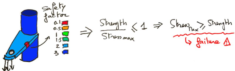
When the stress in the model remains much inferior to the strength of the material, the safety factor stays superior to 1 and the model is « safe ».
