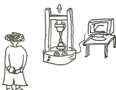
Note that if you need some high accuracy, the test should be performed under conditions similar to the operating conditions of the part or the system (Temperature, strain rate, material grain, flow direction,...)
