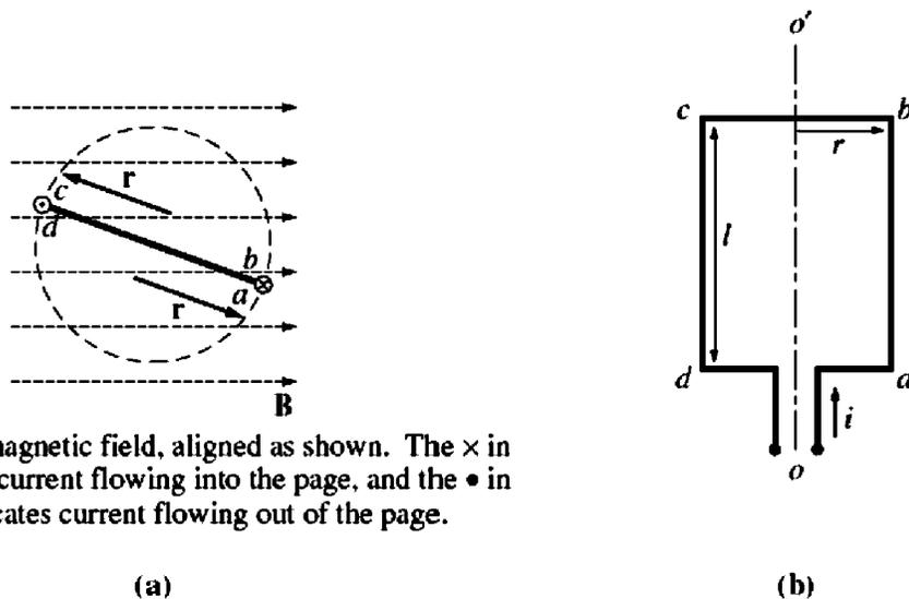
**B** is a uniform magnetic field, aligned as shown. The  $\times$  in a wire indicates current flowing into the page, and the  $\bullet$  in a wire indicates current flowing out of the page.
