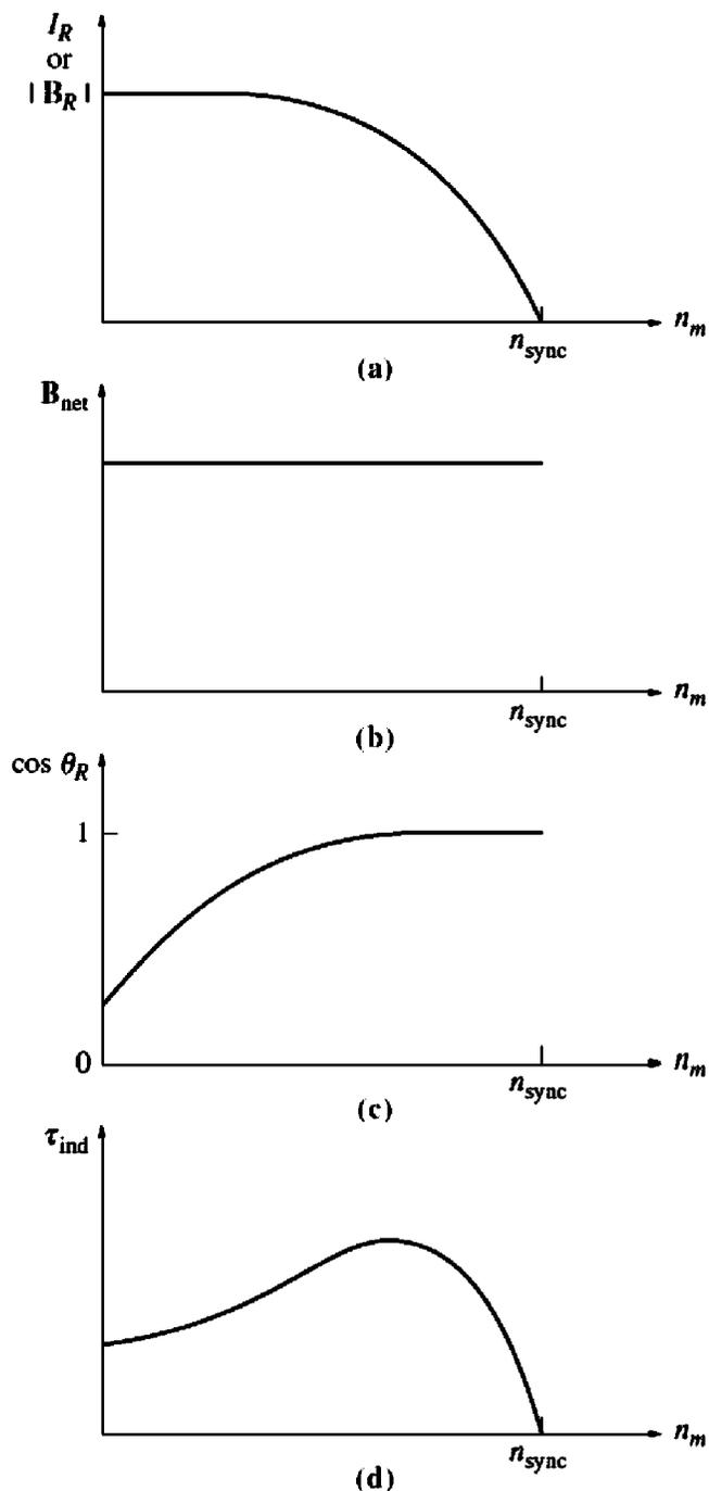
**FIGURE 7-16** Graphical development of an induction motor torque–speed characteristic. (a) Plot of rotor current (and thus  $|B_R|$ ) versus speed for an induction motor; (b) plot of net magnetic field versus speed for the motor; (c) plot of rotor power factor versus speed for the motor; (d) the resulting torque–speed characteristic.
