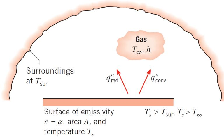
$$G = G_{\text{sur}} = \sigma T_{\text{sur}}^4$$
