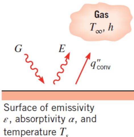
The emissivity of a surface represents the ratio of the radiation emitted by the surface at a given temperature to the radiation emitted by a blackbody at the same temperature.
