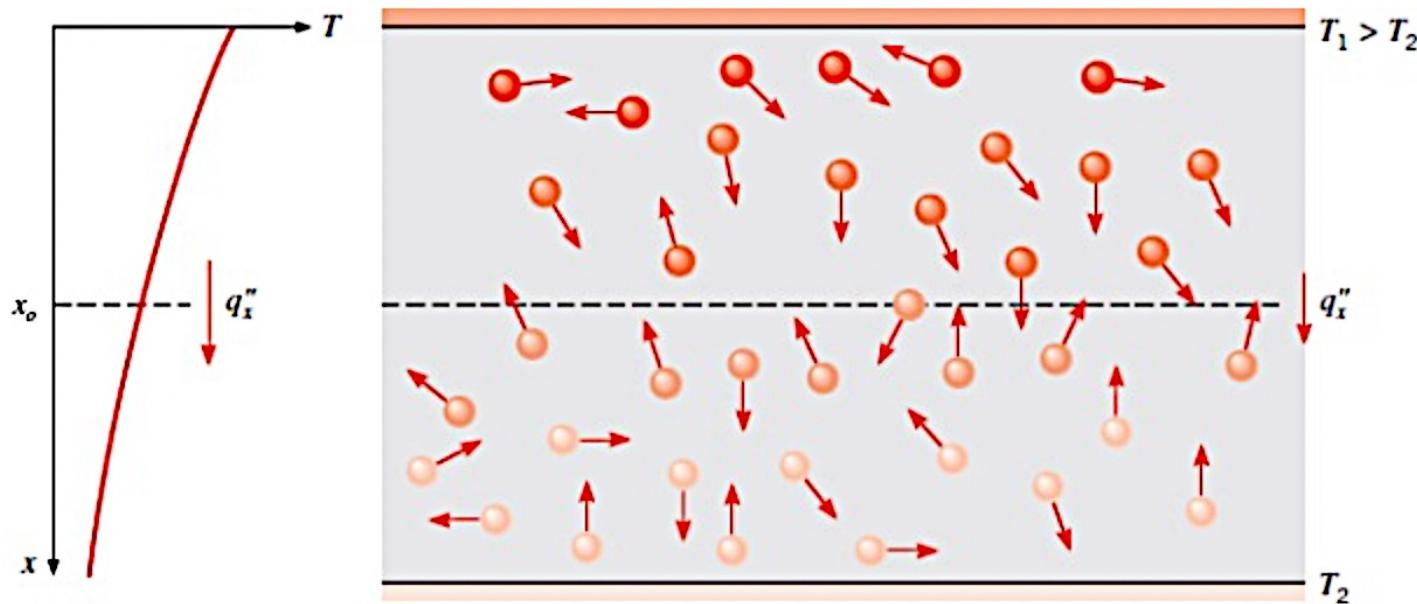
Association of conduction heat transfer with diffusion of energy due to molecular activity
