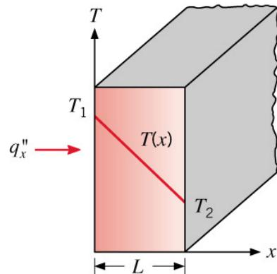
$$q''_x = -k \frac{dT}{dx} = -k \frac{T_2 - T_1}{L}$$
