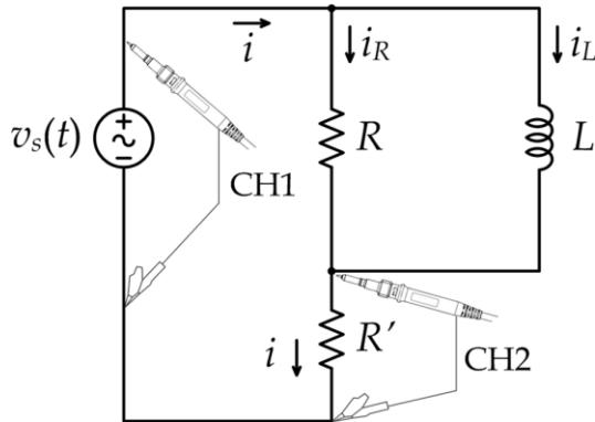
2. Set the function generator to produce a **sinusoidal** waveform (AC) with frequency of **250 Hz**, and peak to peak voltage of  **$V_{pp} = 6 \text{ V}$** .
