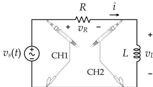
2. Set the function generator to produce a **sinusoidal** waveform (AC) with frequency of **5100 Hz**, and peak to peak voltage of **V<sub>pp</sub> = 6 V**.
