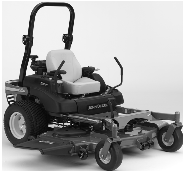
Figure 1-7. Commercial lawn mower with hydrostatic transmission. (Copyright © 1996–2007. All rights reserved. Courtesy of Deere & Company, Cary, North Carolina.)
