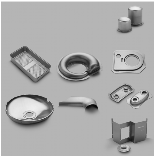
Figure 3-16. Variety of complex shaped parts consisting of different materials, produced by the hydroforming machine of Figure 3-15. (Courtesy of Jones Metal Products Company, West Lafayette, Ohio.)
