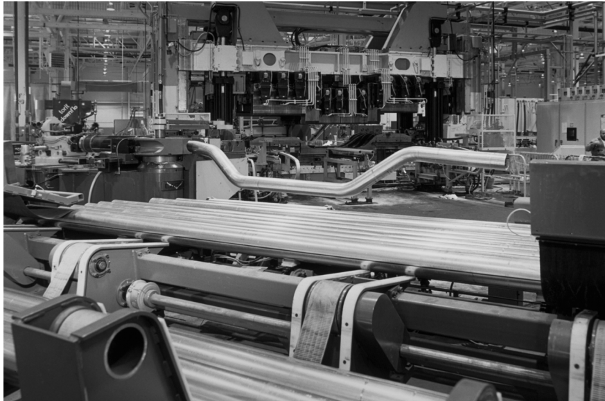
Figure 3-19. Corvette frame rails being produced in factory using tube hydro-forming. (Courtesy of General Motors Corp. Used with permission, GM Media Archives, Detroit, Michigan.)
