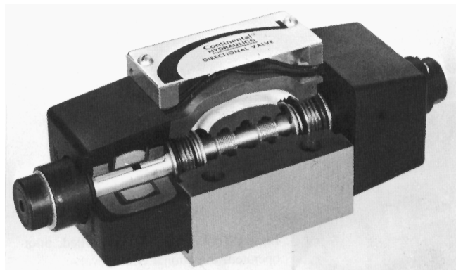
Figure 8-15. Solenoid-actuated, three-position, spring-centered, four-way directional control valve. (Courtesy of Continental Hydraulics, Division of Continental Machines Inc., Savage, Minnesota.)
