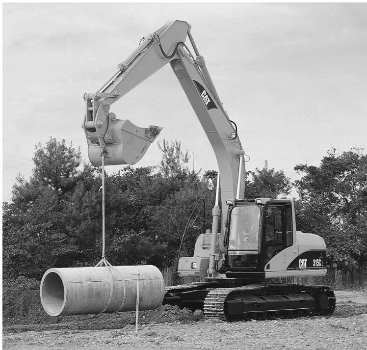
Figure 6-15. Excavator contains hydraulic cylinders whose loadings occur through mechanical linkages. (Courtesy of Caterpillar, Inc., Peoria, Illinois.)
