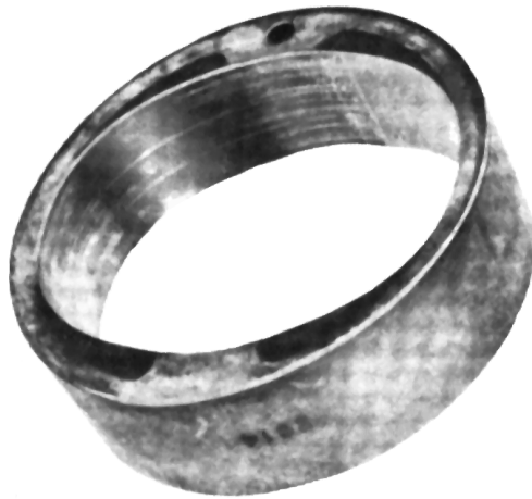
Figure 12-2. Rust caused by moisture in the oil. (Courtesy of Sperry Vickers, Sperry Rand Corp., Troy, Michigan.)
